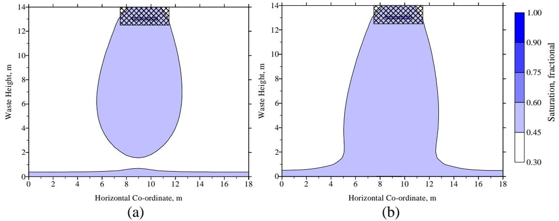
Figure 5.3.4. Predicted saturation iso-clines for a Yolo County Demonstration Project trench after three (a) and four (b) weeks of operation. Daily application rates are shown in Table 5.3.2.
