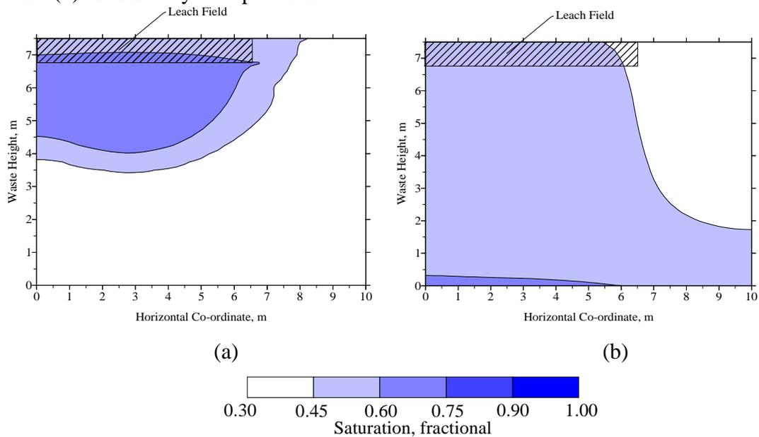
Figure 5.2.6. Saturation iso-clines for waste permeabilities of  $8.1 \times 10^{-3}$  cm/s (a) and 0.1 cm/s (b) after 30 days of operation.
