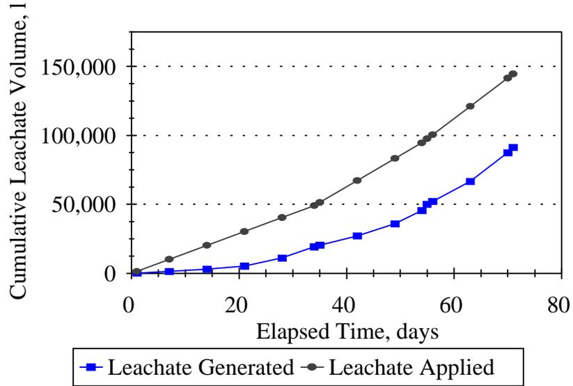
Figure 5.3.1. Cumulative leachate volumes simulated for the Yolo County Project based on an initial saturation of 40%.
