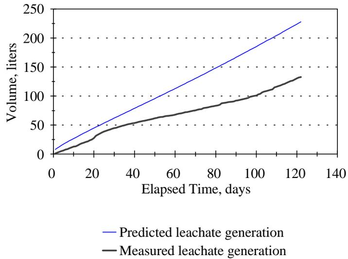
Figure 5.1.1. Predicted and measured leachate generation rates for the Mill Seat pressurized leachate recirculation loop system.
