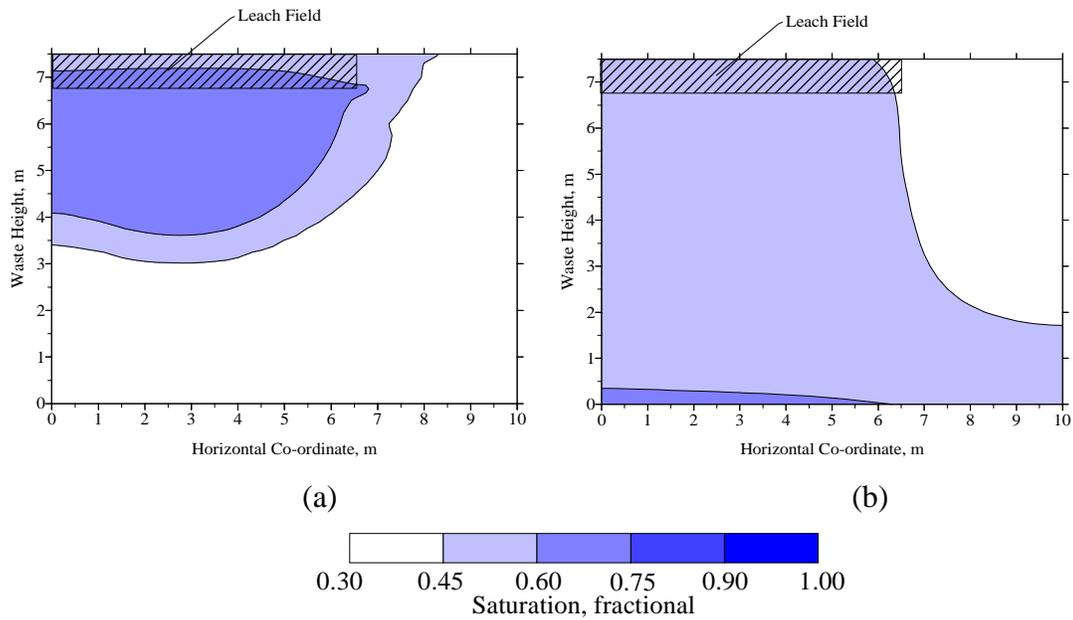
Figure 5.2.7. Saturation iso-clines for waste permeabilities of  $8.1 \times 10^{-3}$  cm/s (a) and 0.1 cm/s (b) after 35 days of operation.
