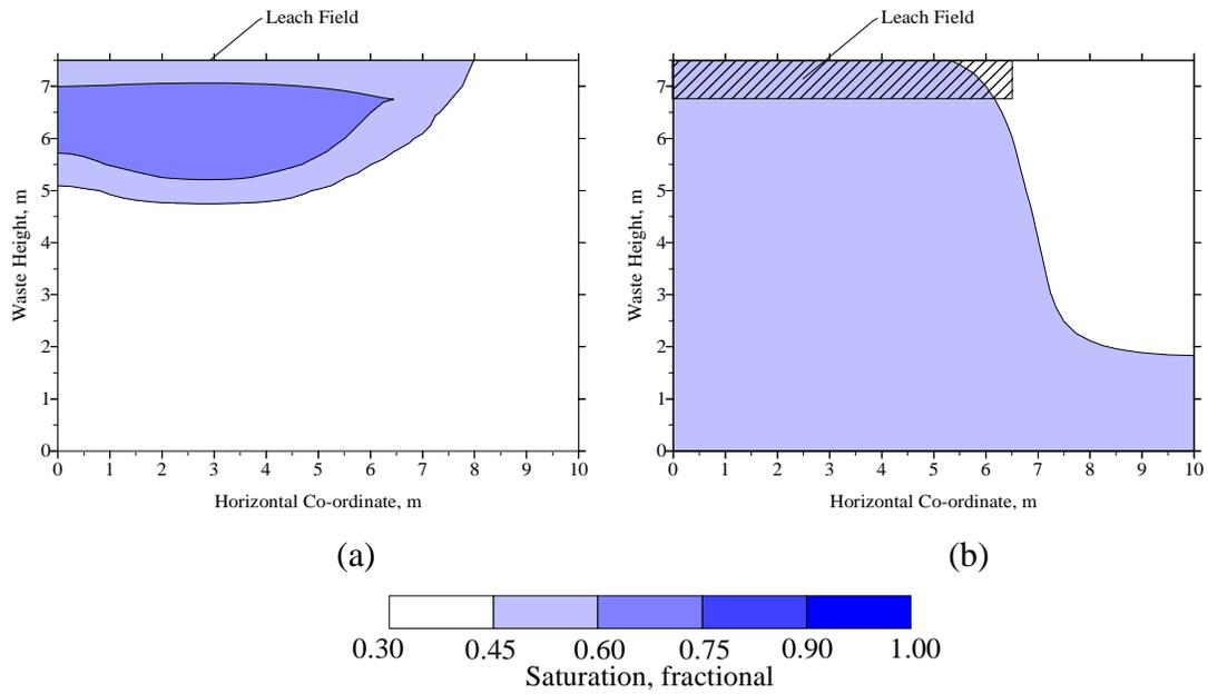
Figure 5.2.3. Saturation iso-clines for waste permeabilities of  $8.1 \times 10^{-3}$  cm/s (a) and 0.1 cm/s (b) after 15 days of operation.
