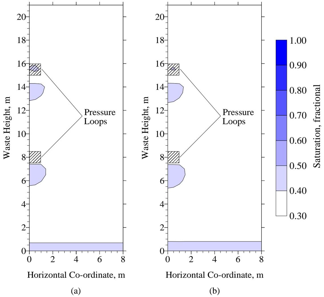
Figure 5.1.4. Saturation iso-clines for the Mill Seat Landfill pressure loop leachate recirculation system at elapsed times of 50 (a) and 60 (b) days.
