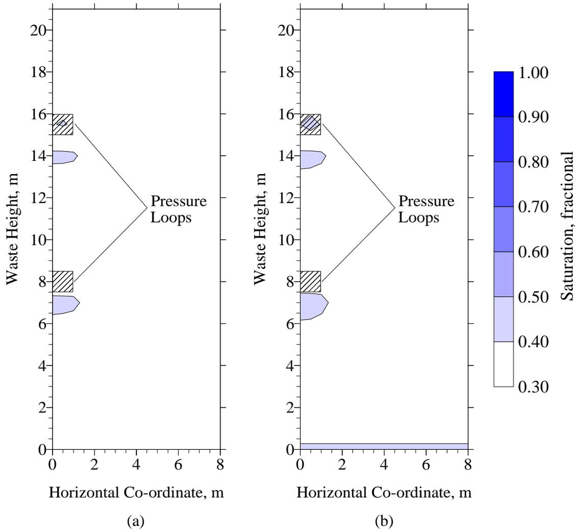
Figure 5.1.2. Saturation iso-clines for the Mill Seat Landfill pressure loop leachate recirculation system at elapsed times of 10 (a) and 20 (b) days.
