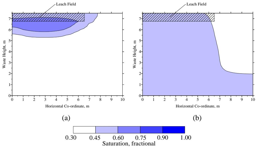
Figure 5.2.2. Saturation iso-clines for waste permeabilities of  $8.1 \times 10^{-3}$  cm/s (a) and 0.1 cm/s (b) after 10 days of operation.
