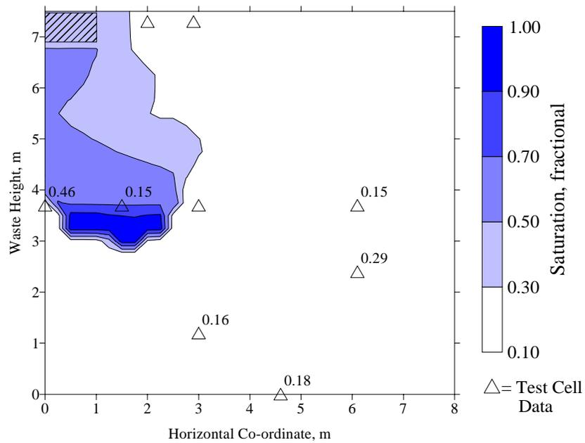
Figure 5.4.6. Simulated saturation iso-clines and measured saturations for the UCF/EPA test cell after six weeks of operation.
