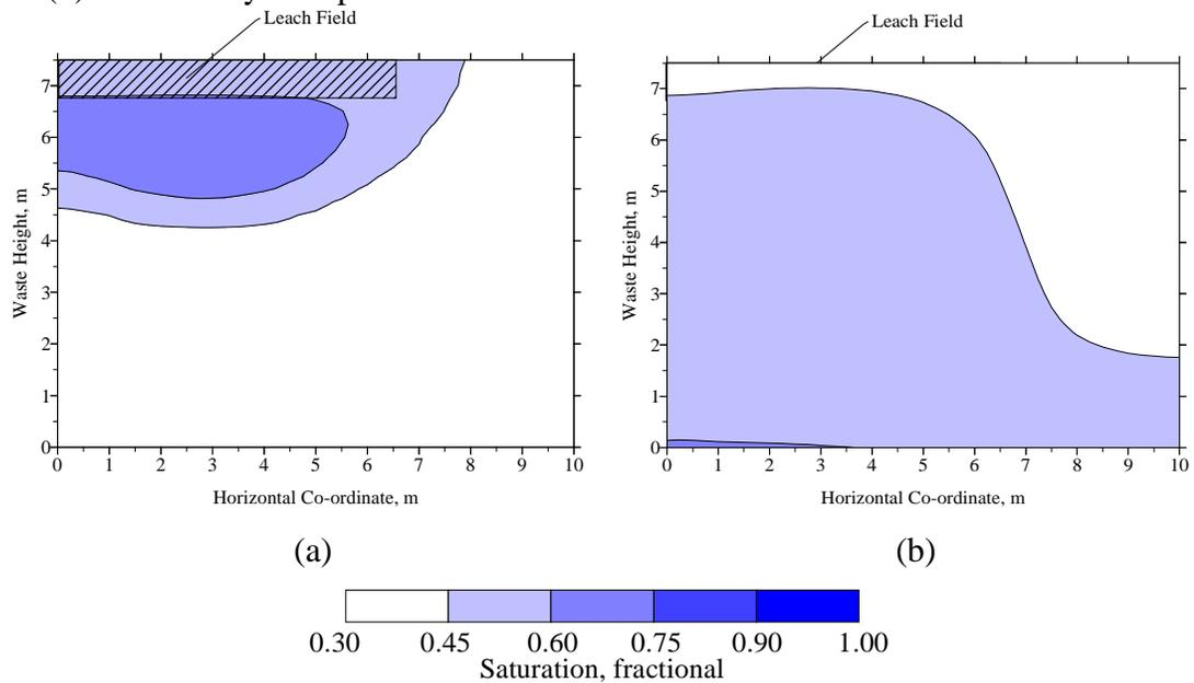
Figure 5.2.4. Saturation iso-clines for waste permeabilities of  $8.1 \times 10^{-3}$  cm/s (a) and 0.1 cm/s (b) after 20 days of operation.
