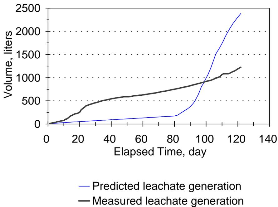
Figure 5.1.8. Predicted and measured leachate generation rates for the Mill Seat deep trench leachate recirculation system.
