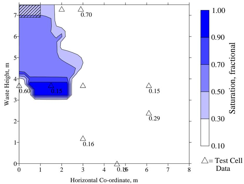
Figure 5.4.4. Simulated saturation iso-clines and measured saturations for the UCF/EPA test cell after four weeks of operation.
