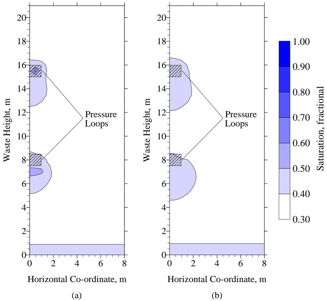
Figure 5.1.5. Saturation iso-clines for the Mill Seat Landfill pressure loop leachate recirculation system at elapsed times of 70 (a) and 80 (b) days.
