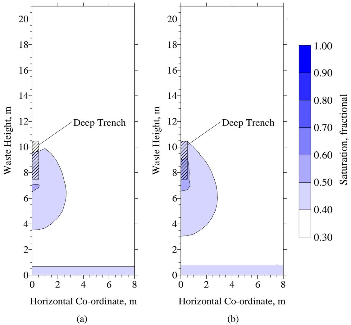
Figure 5.1.11. Saturation iso-clines for the Mill Seat Landfill deep trench leachate recirculation system at elapsed times of 50 (a) and 60 (b) days.
