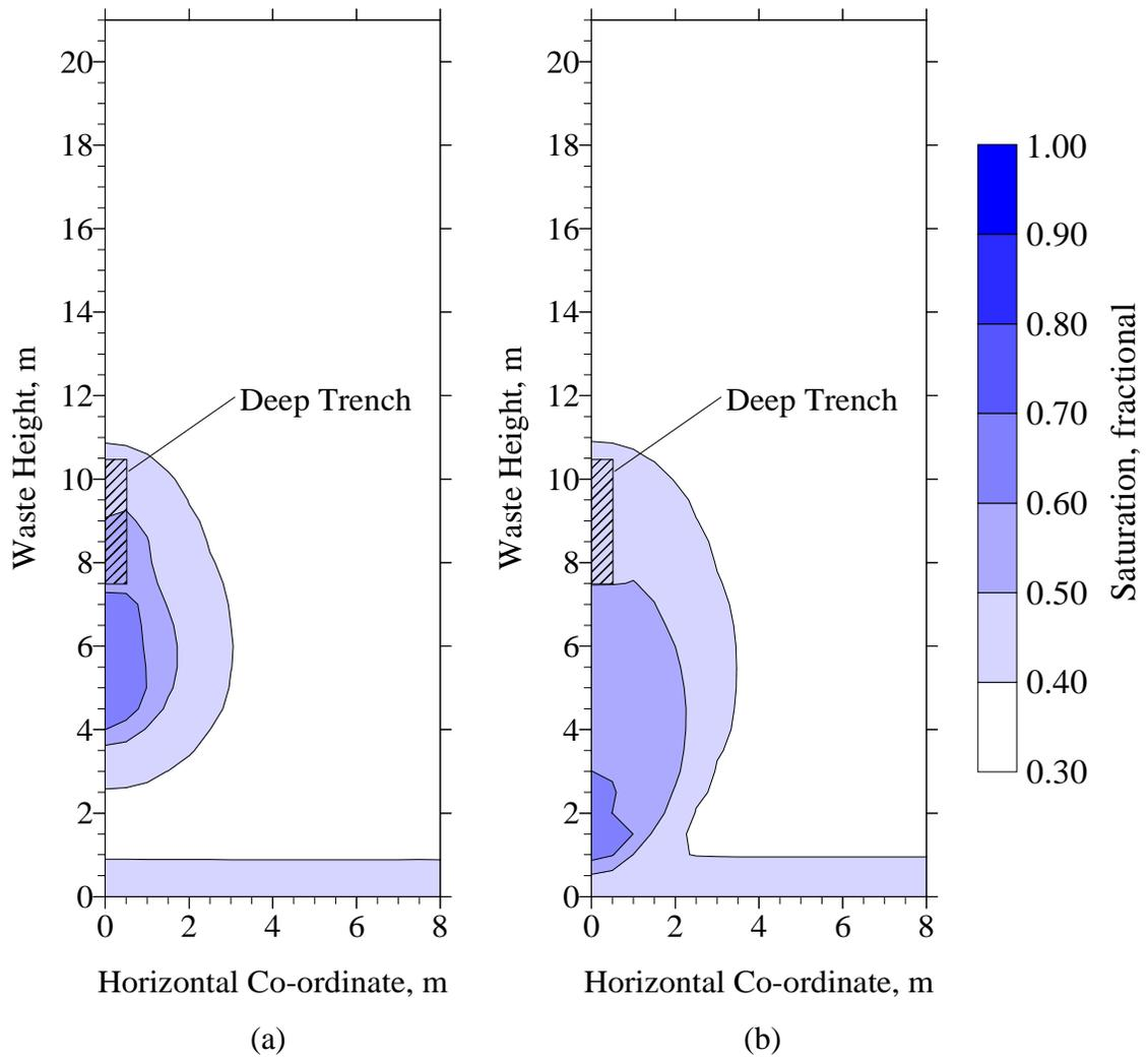
Figure 5.1.12. Saturation iso-clines for the Mill Seat Landfill deep trench leachate recirculation system at elapsed times of 70 (a) and 80 (b) days.
