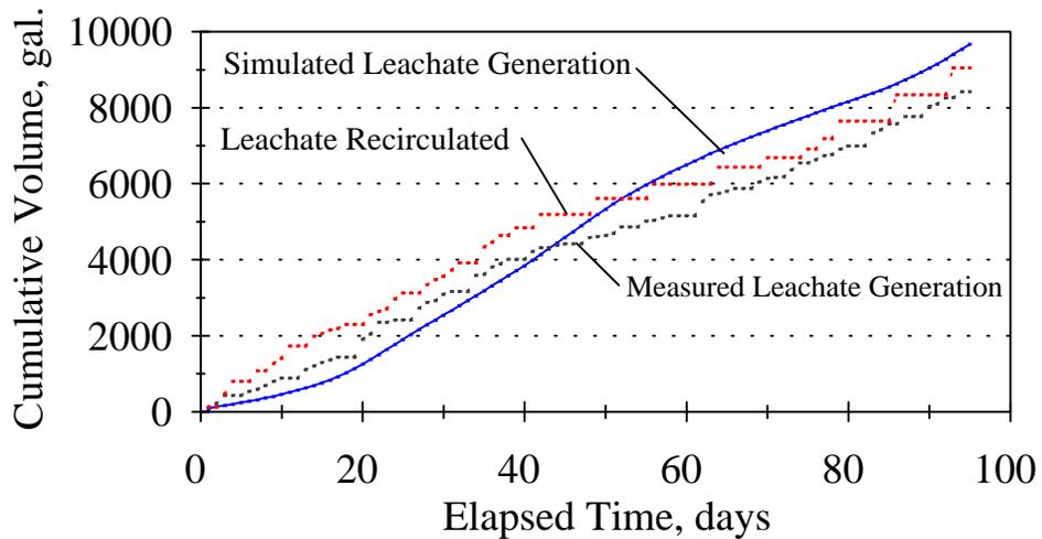
Figure 5.2.9. Cumulative leachate volumes versus time for the DSWA's recirculation test cell.
