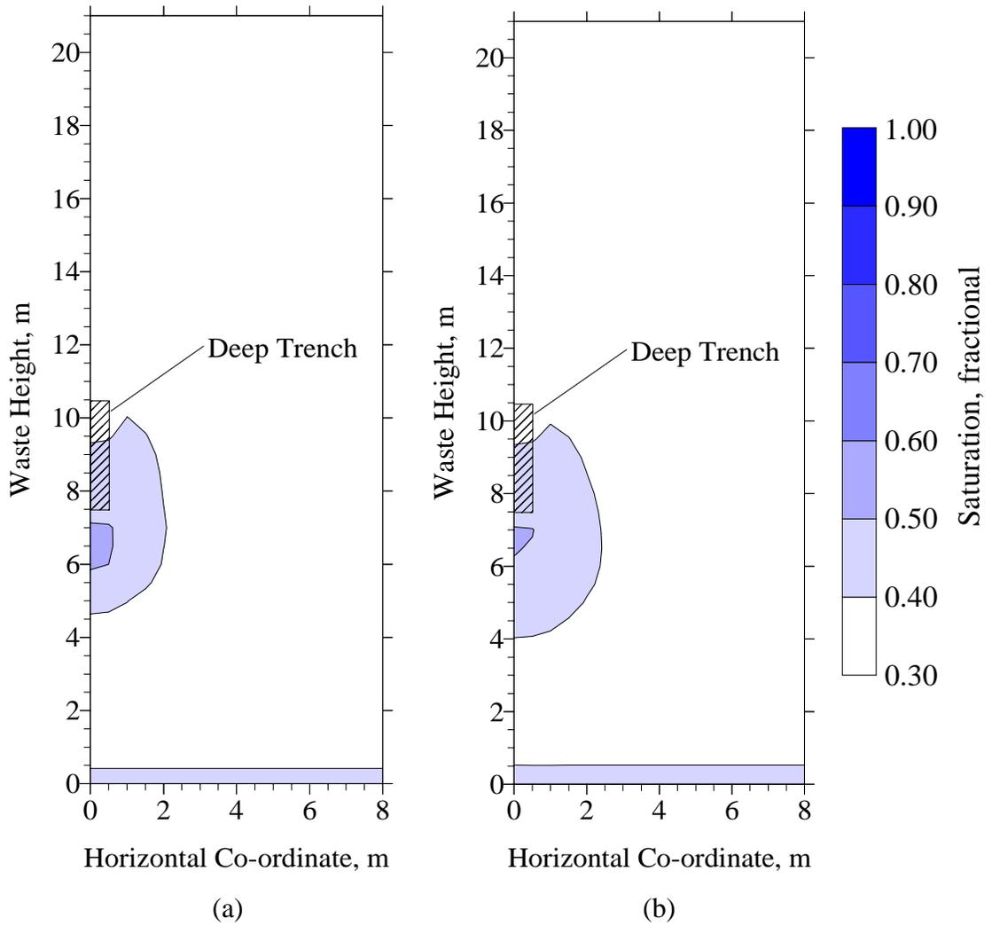
Figure 5.1.10. Saturation iso-clines for the Mill Seat Landfill deep trench leachate recirculation system at elapsed times of 30 (a) and 40 (b) days.
