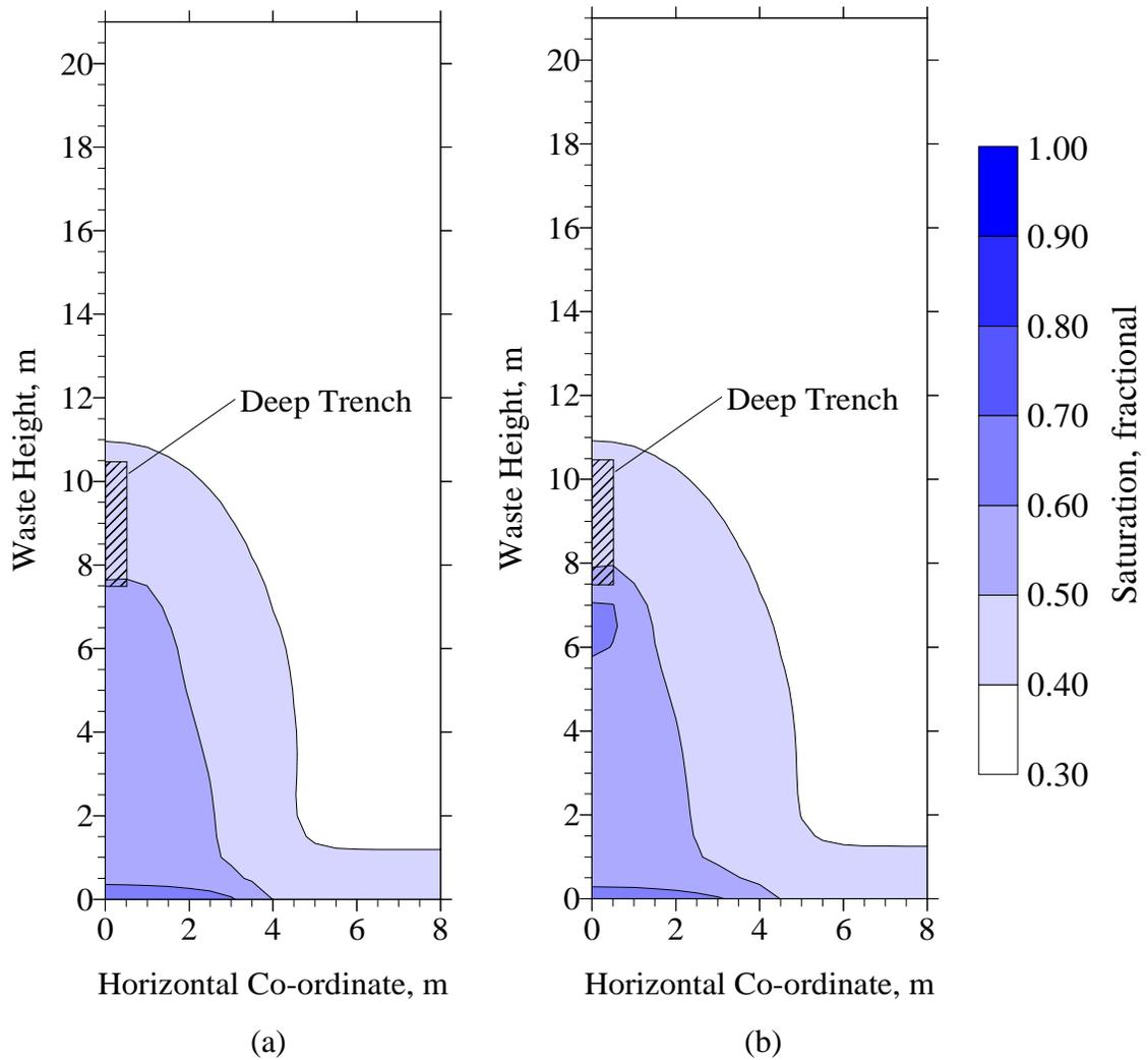
Figure 5.1.14. Saturation iso-clines for the Mill Seat Landfill deep trench leachate recirculation system at elapsed times of 110 (a) and 120 (b) days.
