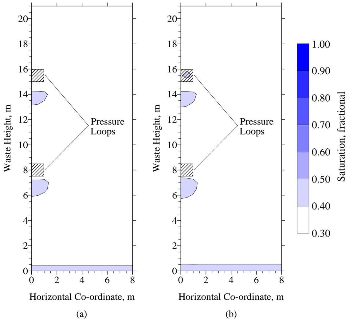
Figure 5.1.3. Saturation iso-clines for the Mill Seat Landfill pressure loop leachate recirculation system at elapsed times of 30 (a) and 40 (b) days.
