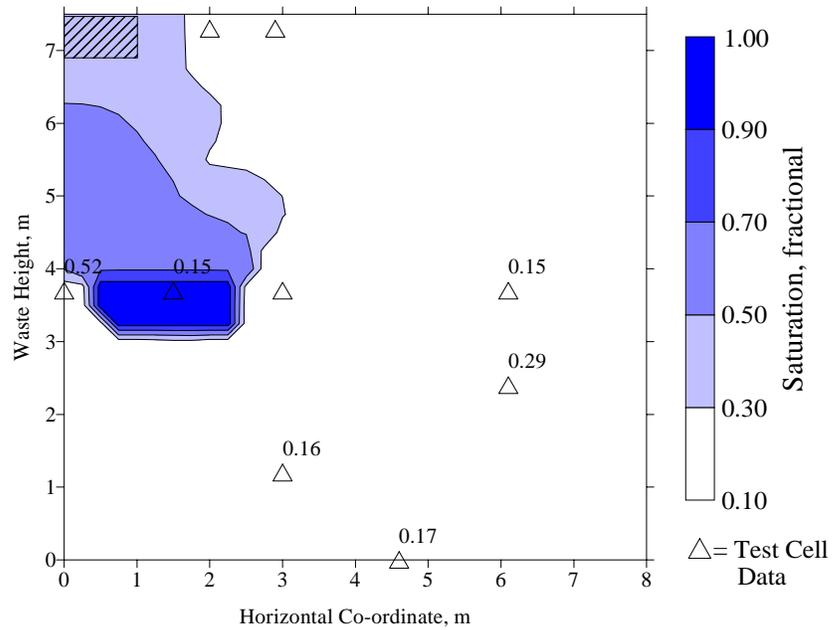
Figure 5.4.5. Simulated saturation iso-clines and measured saturations for the UCF/EPA test cell after five weeks of operation.
