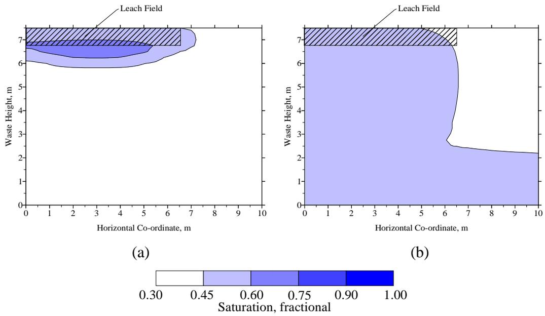
Figure 5.2.1. Saturation iso-clines for waste permeabilities of  $8.1 \times 10^{-3}$  cm/s (a) and 0.1 cm/s (b) after five days of operation.
