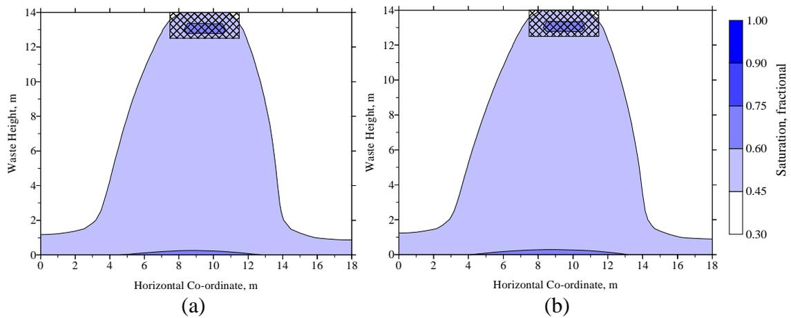
Figure 5.3.7. Predicted saturation iso-clines for a Yolo County Demonstration Project trench after nine (a) and ten (b) weeks of operation. Daily application rates are shown in Table 5.3.2.
