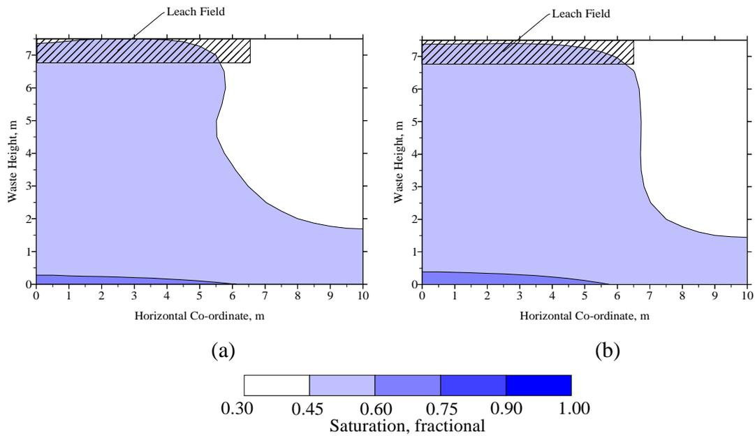
Figure 5.2.8. Saturation iso-clines for a waste permeability of 0.1 cm/s after 65 (a) and 95 (b) days of operation.
