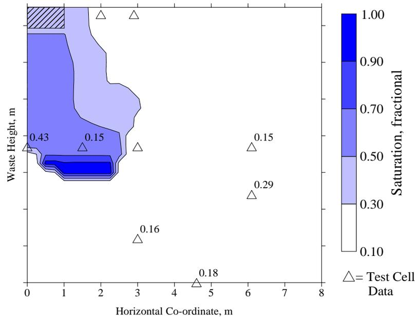
Figure 5.4.7. Simulated saturation iso-clines and measured saturations for the UCF/EPA test cell after seven weeks of operation.
