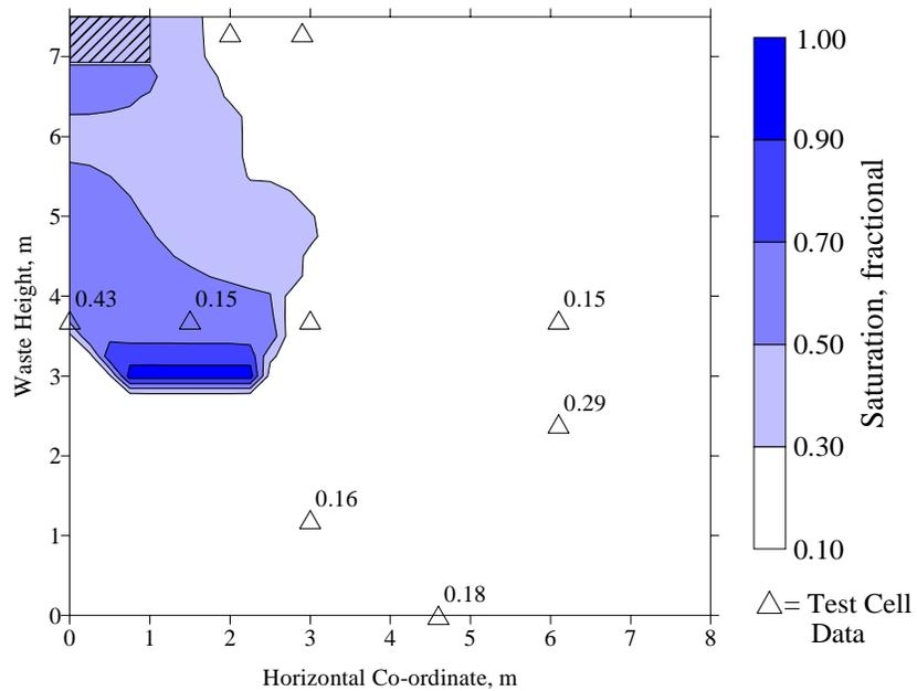
Figure 5.4.8. Simulated saturation iso-clines and measured saturations for the UCF/EPA test cell after eight weeks of operation.
