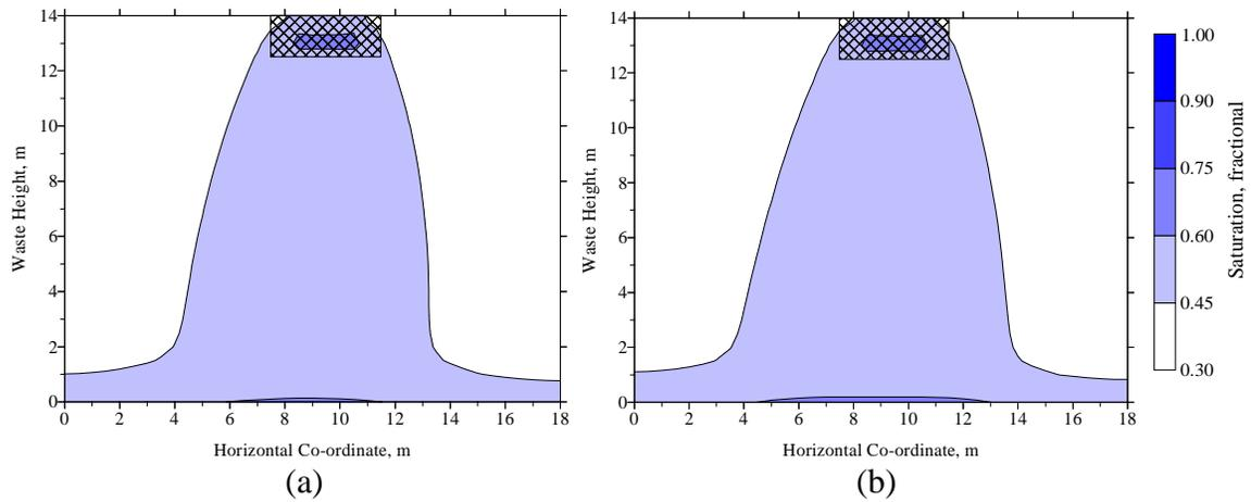
Figure 5.3.6. Predicted saturation iso-clines for a Yolo County Demonstration Project trench after seven (a) and eight (b) weeks of operation. Daily application rates are shown in Table 5.3.2.
