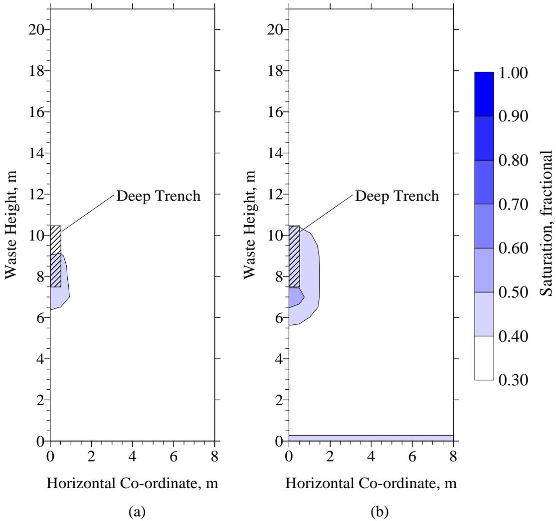
Figure 5.1.9. Saturation iso-clines for the Mill Seat Landfill deep trench leachate recirculation system at elapsed times of 10 (a) and 20 (b) days.
