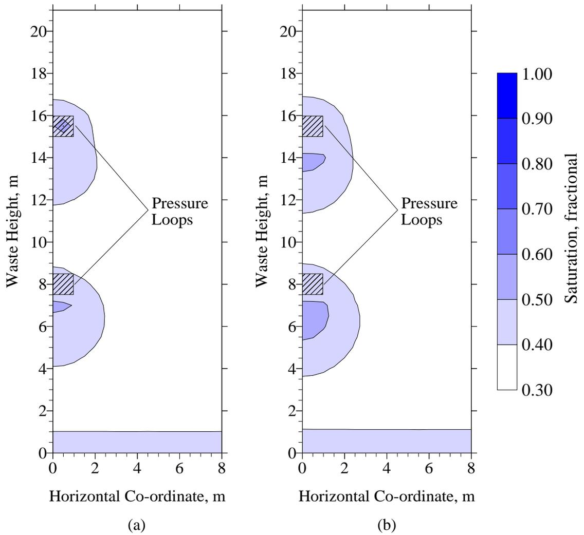
Figure 5.1.6. Saturation iso-clines for the Mill Seat Landfill pressure loop leachate recirculation system at elapsed times of 90 (a) and 100 (b) days.
