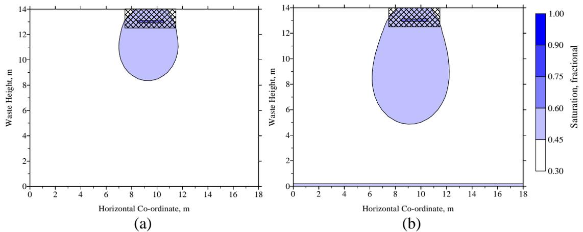
Figure 5.3.3. Predicted saturation iso-clines for a Yolo County Demonstration Project trench after one (a) and two (b) weeks of operation. Daily application rates are shown in Table 5.3.2.
