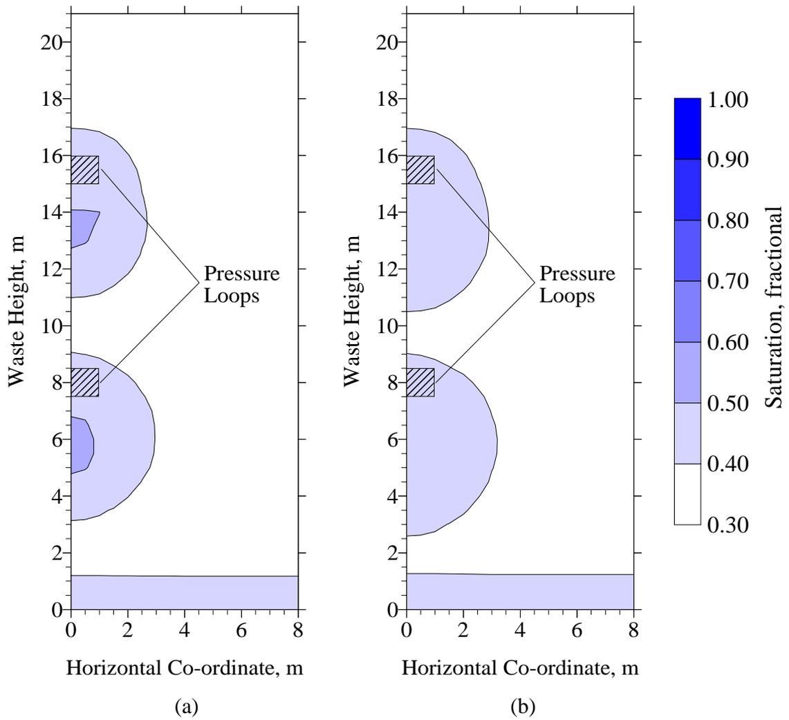
Figure 5.1.7. Saturation iso-clines for the Mill Seat Landfill pressure loop leachate recirculation system at elapsed times of 110 (a) and 120 (b) days.
