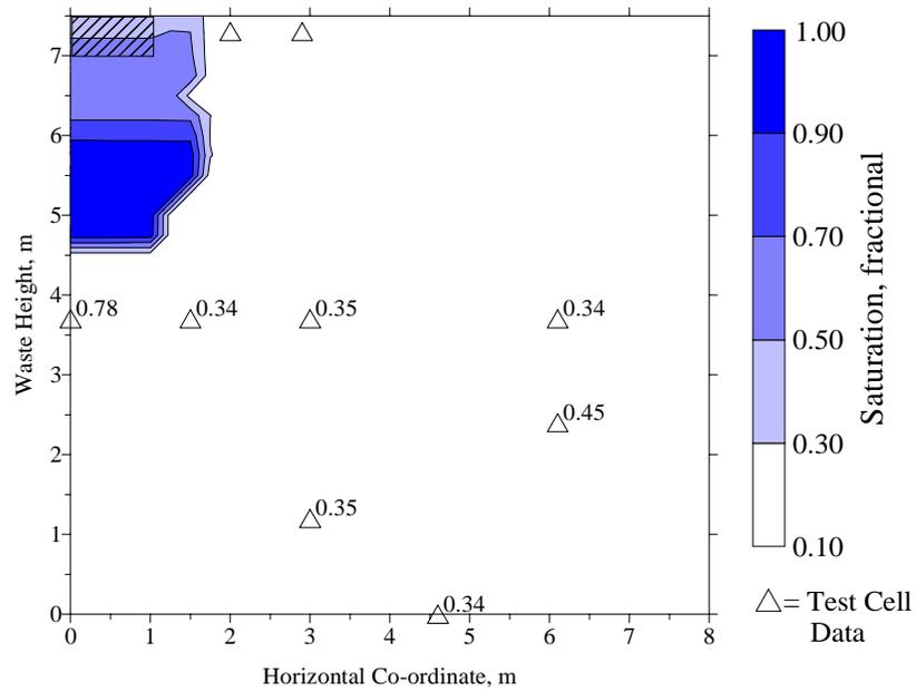
Figure 5.4.1. Simulated saturation iso-clines and measured saturations for the UCF/EPA test cell after one week of operation.
