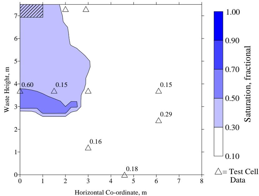
Figure 5.4.9. Simulated saturation iso-clines and measured saturations for the UCF/EPA test cell after thirteen weeks of operation.
