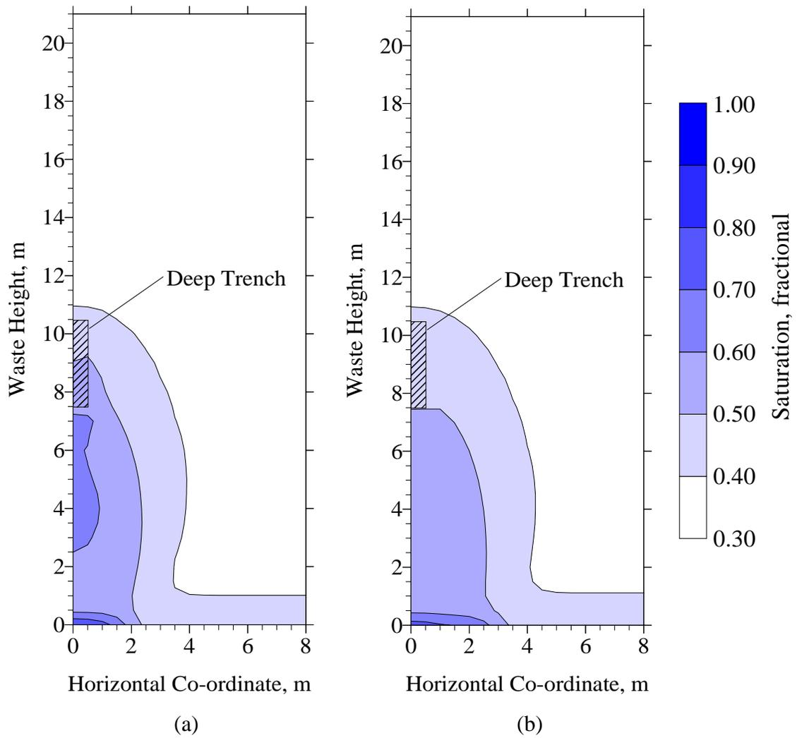
Figure 5.1.13. Saturation iso-clines for the Mill Seat Landfill deep trench leachate recirculation system at elapsed times of 90 (a) and 100 (b) days.
