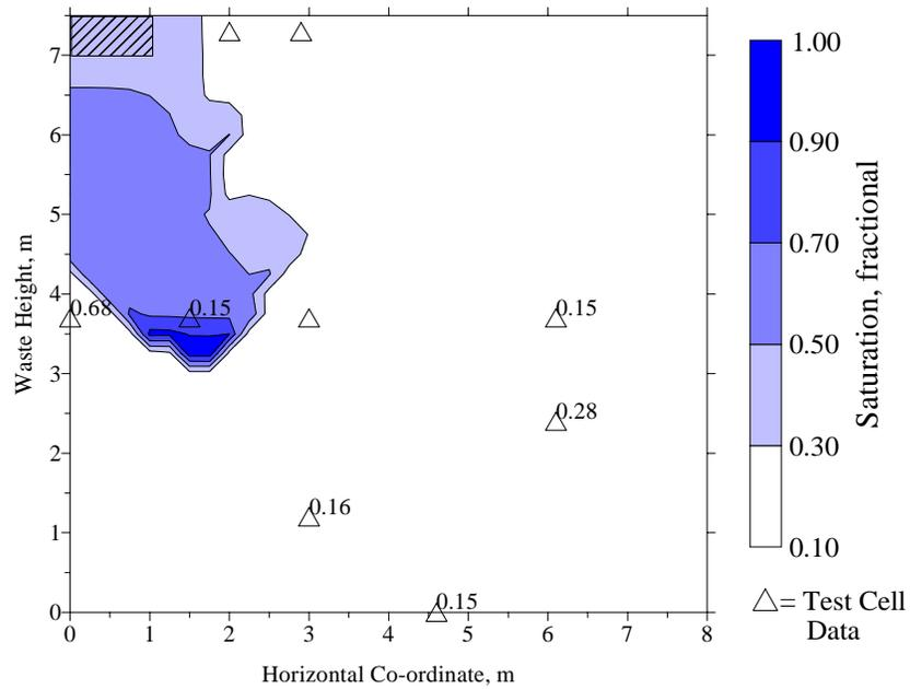
Figure 5.4.3. Simulated saturation iso-clines and measured saturations for the UCF/EPA test cell after three weeks of operation.
