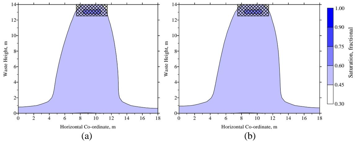
Figure 5.3.5. Predicted saturation iso-clines for a Yolo County Demonstration Project trench after five (a) and six (b) weeks of operation. Daily application rates are shown in Table 5.3.2.
