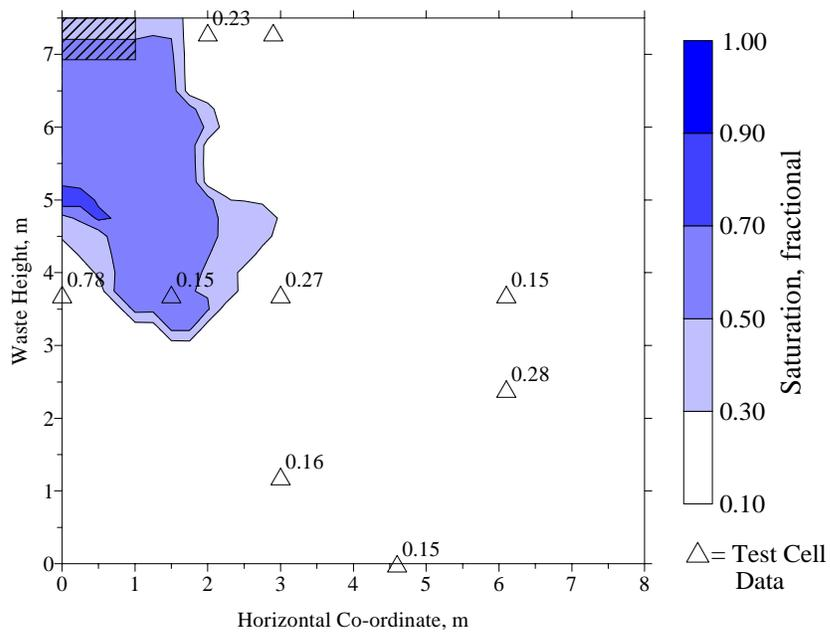
Figure 5.4.2. Simulated saturation iso-clines and measured saturations for the UCF/EPA test cell after two weeks of operation.
