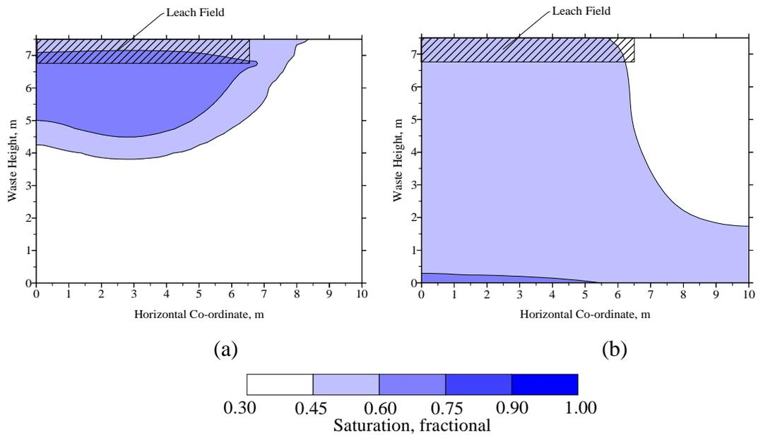
Figure 5.2.5. Saturation iso-clines for waste permeabilities of  $8.1 \times 10^{-3}$  cm/s (a) and 0.1 cm/s (b) after 25 days of operation.
