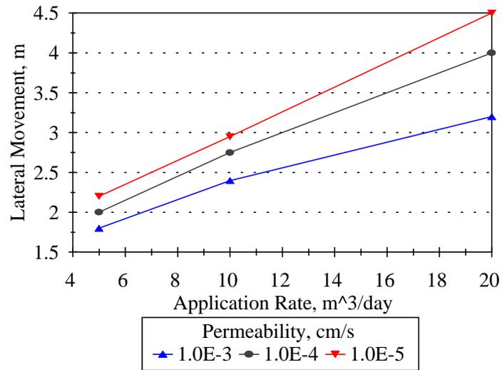
Figure 4.2.9. Lateral movement versus flow rate after two weeks of intermittent leachate application (8 hr on/16 hr off).
