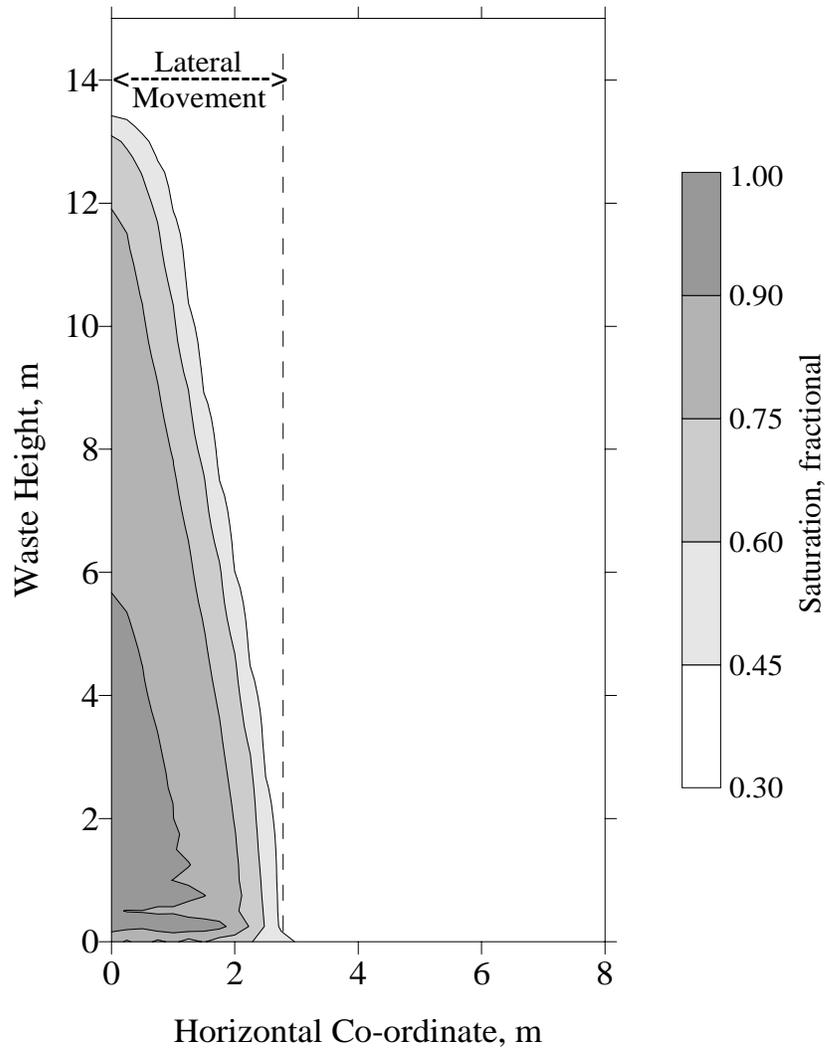
Figure 4.2.1. Calculation of lateral movement, leachate applied intermittently (8 hr on/16 hr off) at  $10 \text{ m}^3/\text{m}/\text{day}$  for three weeks, waste permeability =  $1 \times 10^{-3} \text{ cm/s}$ .
