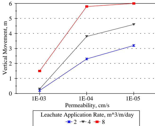
Figure 4.1.3. Maximum upward movement versus permeability for constant leachate injection.
