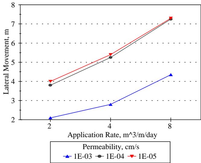
Figure 4.1.4. Lateral Movement Versus Flow Rate for Constant Leachate Injection.
