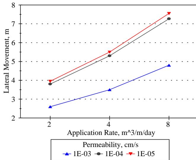
Figure 4.1.9. Lateral Movement Versus Flow Rate for Intermittent Leachate Injection (8 hr on/16 hr off).
