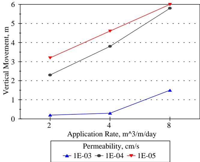
Figure 4.1.5. Upward Movement Versus Flow Rate for Constant Leachate Injection.
