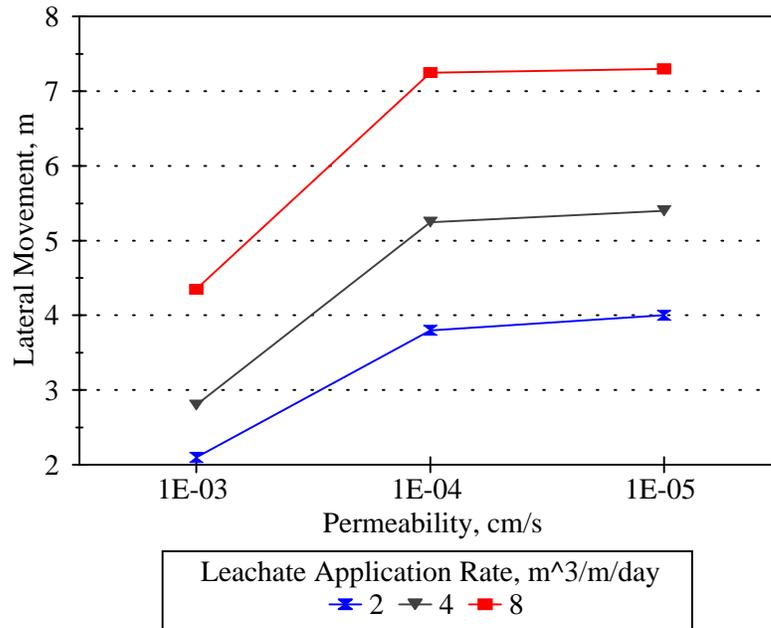
Figure 4.1.2. Maximum lateral movement versus permeability for constant leachate injection.
