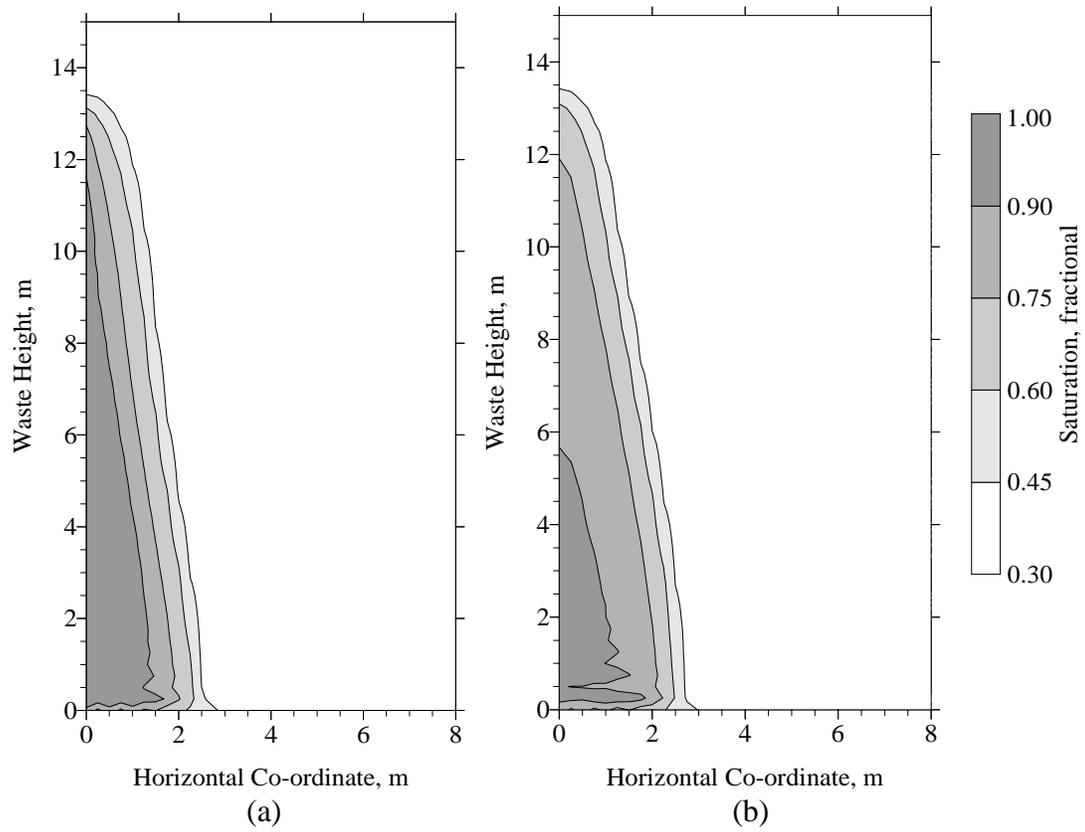
Figure 4.2.12. Saturation iso-clines for the vertical well operated constantly (a) and intermittently (b) at an average rate of  $10 \text{ m}^3/\text{day}$  for three weeks. Waste permeability =  $10^{-3} \text{ cm/s}$ .
