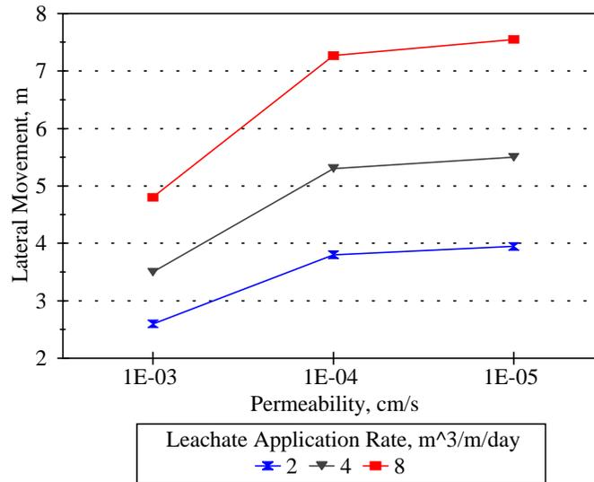
Figure 4.1.7. Maximum lateral movement versus permeability for intermittent leachate injection (8 hr on/16 hr off).
