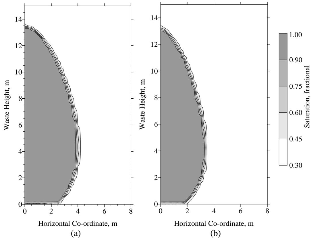
Figure 4.2.13. Saturation iso-clines for the vertical well operated constantly (a) and intermittently (b) at an average rate of  $10 \text{ m}^3/\text{day}$  for three weeks. Waste permeability =  $10^{-5} \text{ cm/s}$ .
