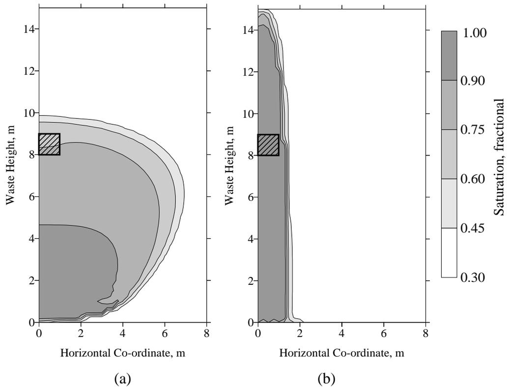
Figure 4.4.1. Leachate routing for an anisotropic waste mass with a longitudinal permeability of  $10^{-3}$  cm/s and a transverse permeability of  $10^{-2}$  cm/s (a) or  $10^{-4}$  cm/s (b) after one week of operation. Leachate applied 8 hr per day at a rate of  $4 \text{ m}^3/\text{m}$  of trench/day.
