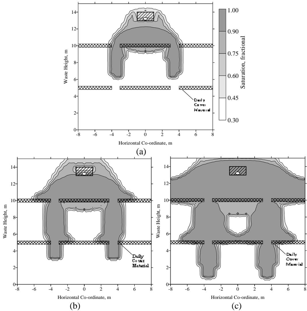
Figure 4.3.1. Comparison of leachate routing in a landfill with a low permeability daily cover material (permeability =  $10^{-5}$  cm/s) with intermittent leachate application at a daily rate of 2, 4, and 8  $\text{m}^3/\text{m}/\text{day}$  (a, b, and c respectively). Waste permeability =  $10^{-3}$  cm/s.
