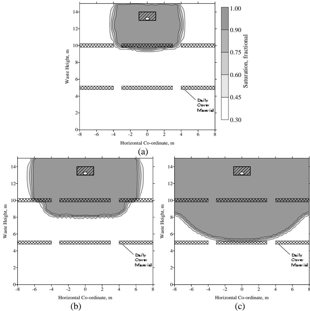
Figure 4.3.4. Comparison of leachate routing in a landfill with a low permeability daily cover material (permeability =  $10^{-5}$  cm/s) with intermittent leachate application at a daily rate of 2, 4, and 8  $\text{m}^3/\text{m}/\text{day}$  (a, b, and c respectively). Waste permeability =  $10^{-4}$  cm/s.
