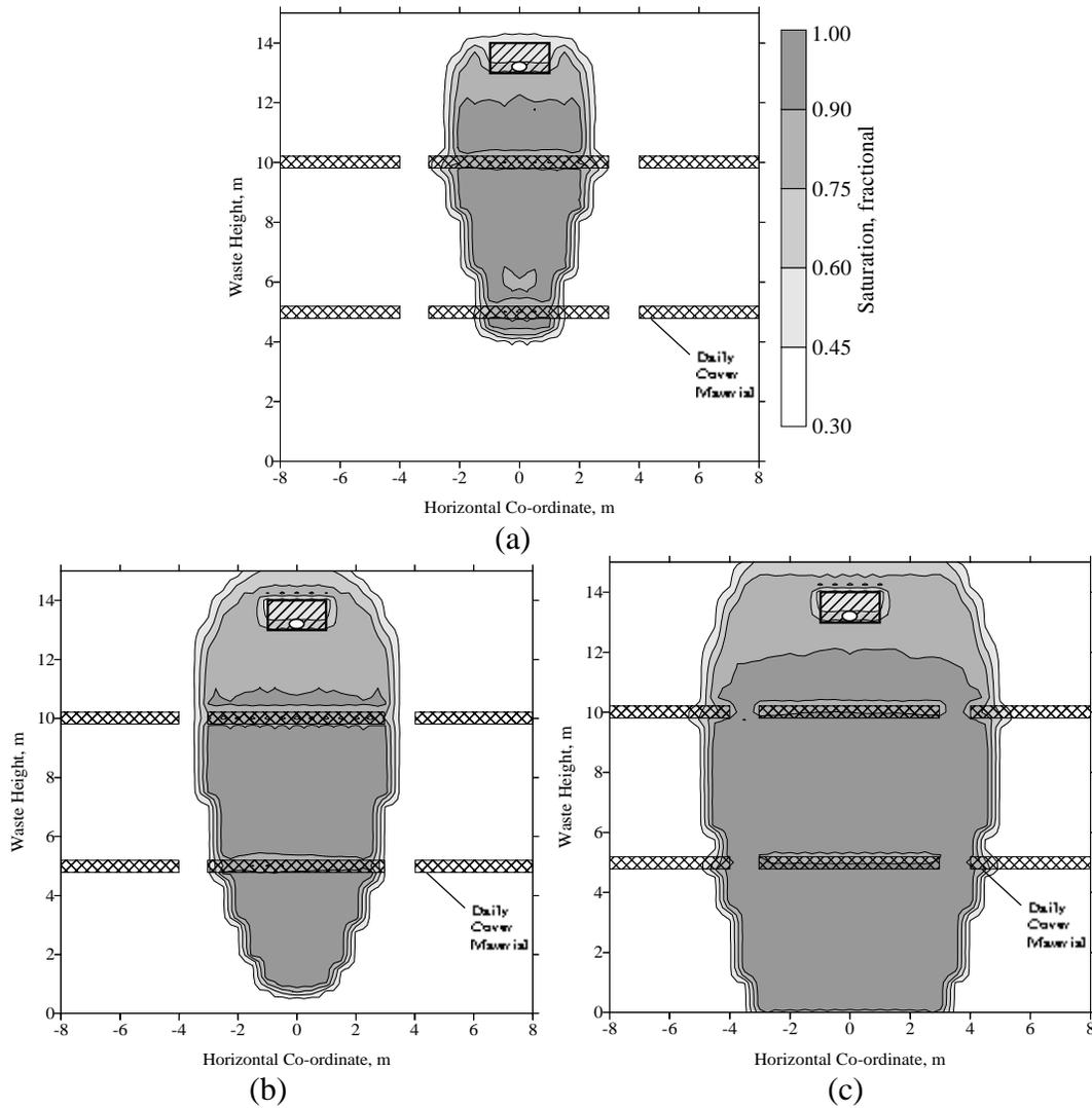
Figure 4.3.3. Comparison of leachate routing in a landfill with a high permeability daily cover material (permeability =  $10^{-2}$  cm/s) with intermittent leachate application at a daily rate of 2, 4, and 8  $\text{m}^3/\text{m}/\text{day}$  (a, b, and c respectively). Waste permeability =  $10^{-3}$  cm/s.
