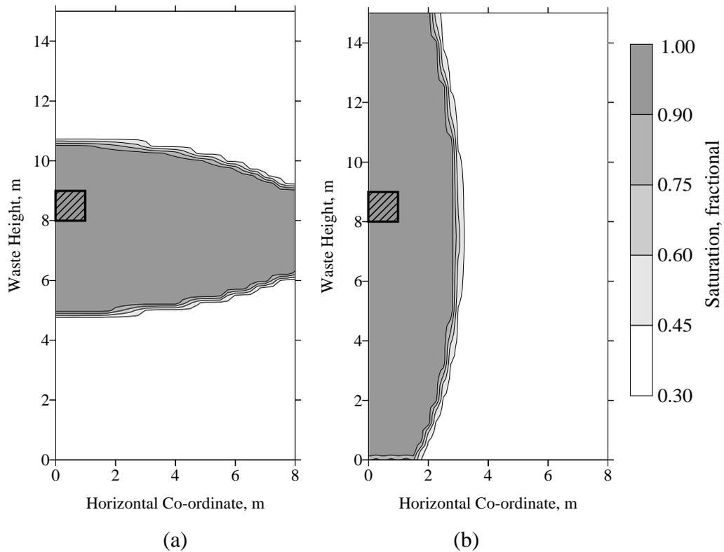
Figure 4.4.2. Leachate routing for an anisotropic waste mass with a longitudinal permeability of  $10^{-4}$  cm/s and a transverse permeability of  $10^{-3}$  cm/s (a) or  $10^{-5}$  cm/s (b) after one week of operation. Leachate applied 8 hr per day at a rate of  $4 \text{ m}^3/\text{m}$  of trench/day.
