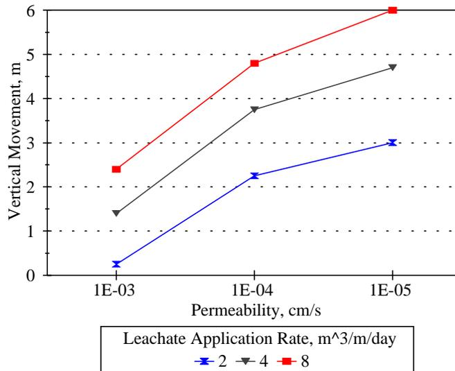
Figure 4.1.8. Maximum upward movement versus permeability for intermittent leachate injection (8 hr on/16 hr off).
