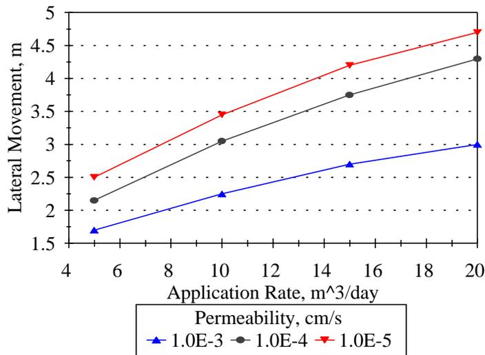
Figure 4.2.4. Lateral movement versus flow rate after two weeks of constant leachate application.
