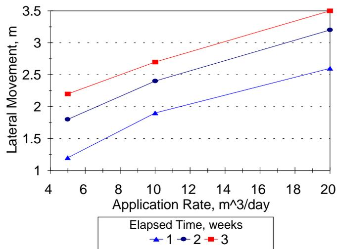
Figure 4.2.7. Lateral movement versus flow rate for one to three weeks of intermittent leachate application (8 hr on/16 hr off) to a waste mass with a permeability of  $10^{-3}$  cm/s.
