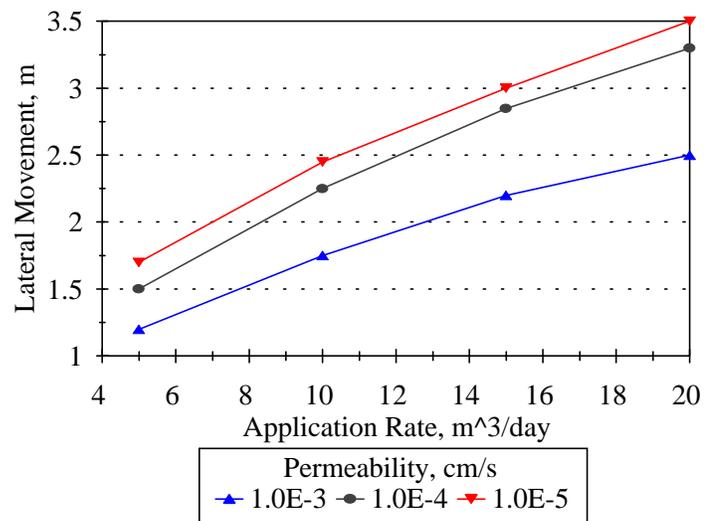
Figure 4.2.3. Lateral movement versus flow rate after one week of constant leachate application.
