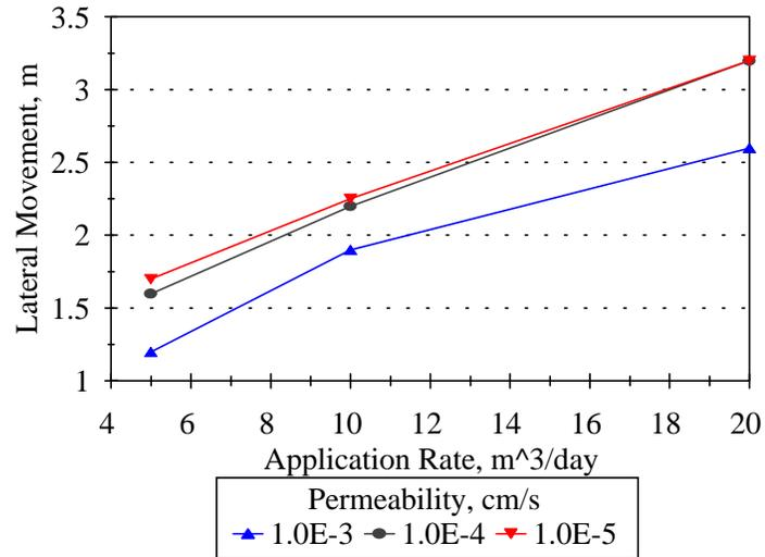
Figure 4.2.8. Lateral movement versus flow rate after one week of intermittent leachate application (8 hr on/16 hr off).
