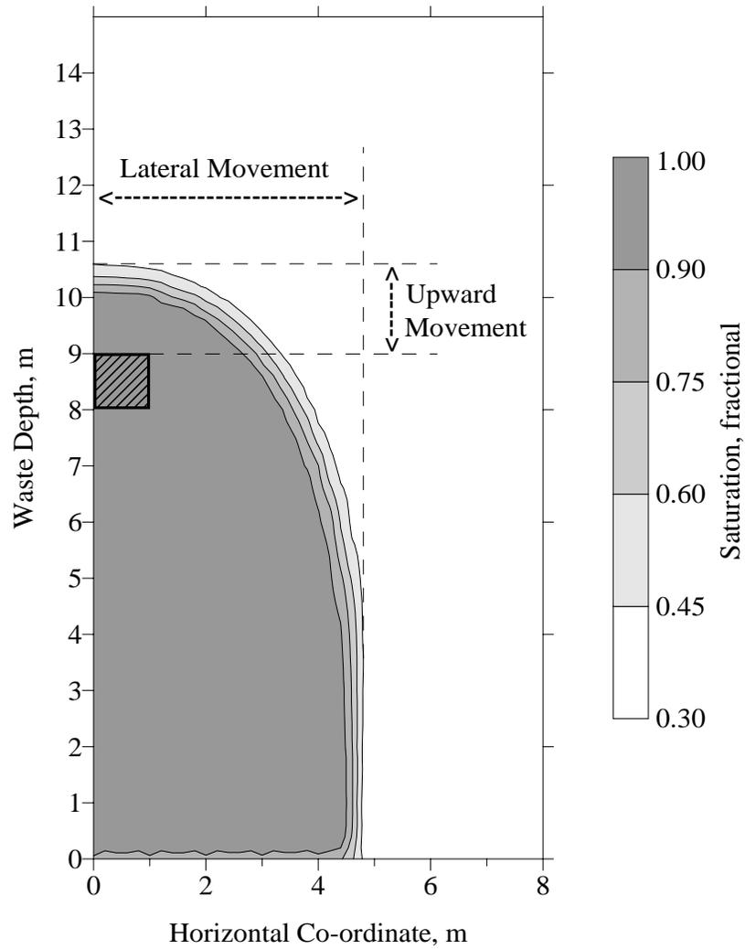
Figure 4.1.1. Schematic depicting the calculation method for the lateral and upward movement, leachate applied continuously at  $8 \text{ m}^3/\text{m}/\text{day}$  for one week, waste permeability  $= 1 \times 10^{-3} \text{ cm/s}$ .
