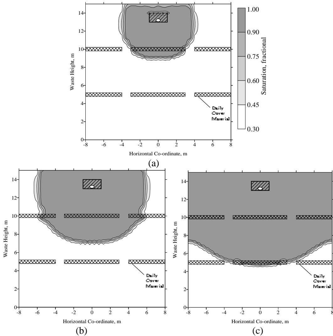
Figure 4.3.5. Comparison of leachate routing in a landfill with a high permeability daily cover material (permeability =  $10^{-3}$  cm/s) with intermittent leachate application at a daily rate of 2, 4, and 8  $\text{m}^3/\text{m}/\text{day}$  (a, b, and c respectively). Waste permeability =  $10^{-4}$  cm/s.
