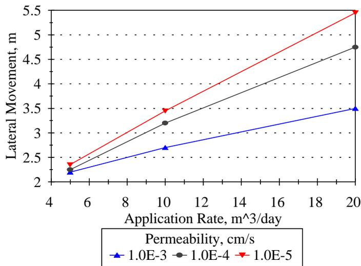
Figure 4.2.10. Lateral movement versus flow rate after three weeks intermittent leachate application (8 hr on/16 hr off).
