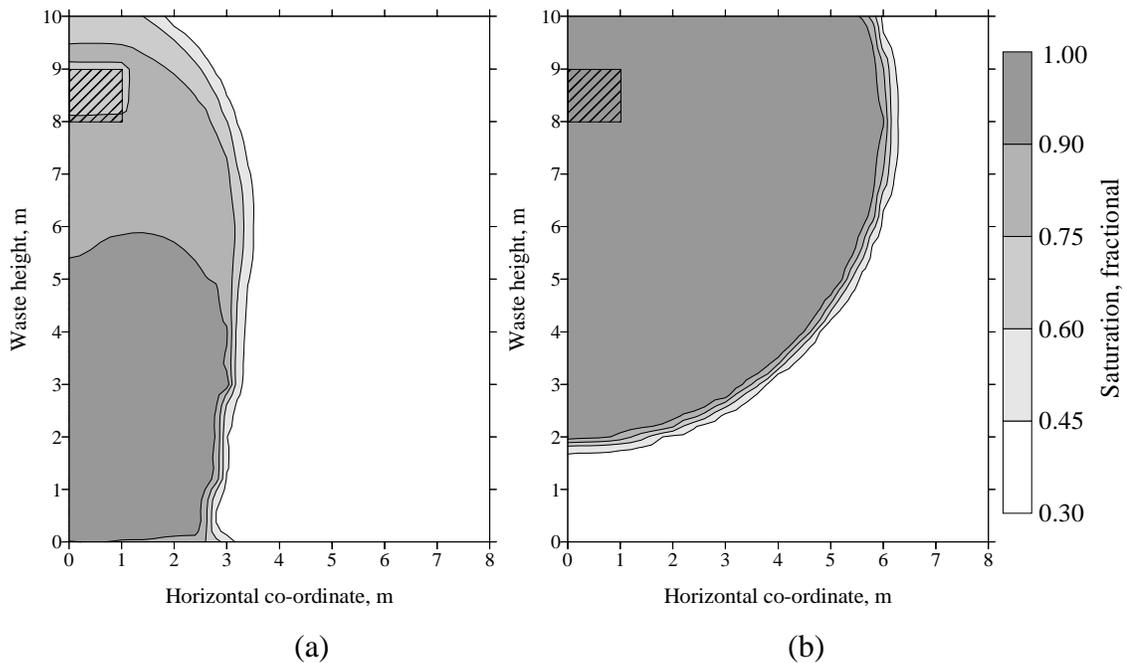
Figure 4.5.1. Comparison of leachate routing for homogeneous waste masses with permeabilities of  $10^{-3}$  (a) and  $10^{-4}$  (b) cm/s after one week of operation. Leachate applied 8 hr per day at a rate of  $4 \text{ m}^3/\text{m}$  of trench/day.
