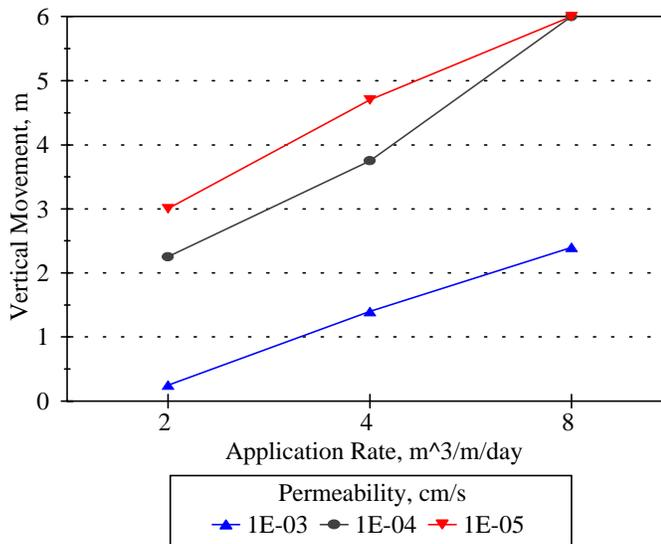
Figure 4.1.10. Upward Movement Versus Flow Rate for Intermittent Leachate Injection (8 hr on/16 hr off).
