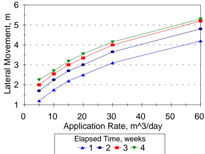
Figure 4.2.2. Lateral movement versus flow rate for one to four weeks of constant leachate application to a waste mass with a permeability of  $10^{-3}$  cm/s.
