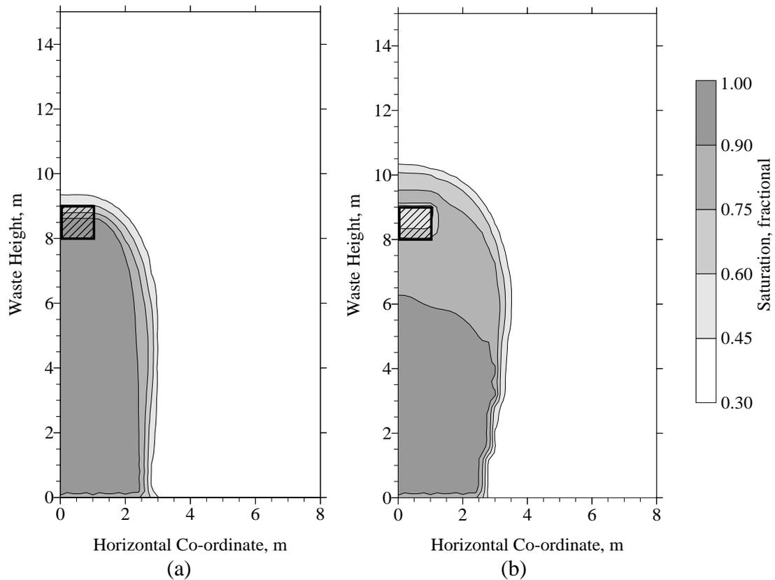
Figure 4.1.12. Saturation iso-clines for the horizontal trench operated constantly (a) and intermittently (b) at an average rate of  $4\text{m}^3/\text{m}/\text{day}$  after one week. Waste permeability =  $10^{-3}$  cm/s.
