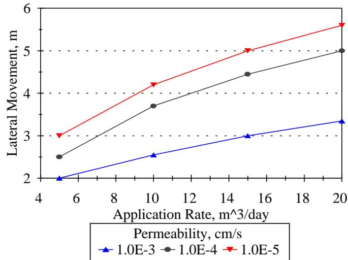
Figure 4.2.5. Lateral movement versus flow rate after three weeks of constant leachate application.
