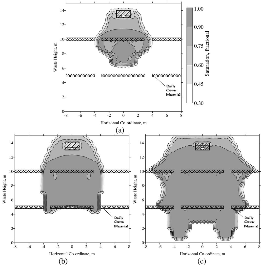
Figure 4.3.2. Comparison of leachate routing in a landfill with a low permeability daily cover material (permeability =  $10^{-4}$  cm/s) with intermittent leachate application at a daily rate of 2, 4, and 8  $\text{m}^3/\text{m}/\text{day}$  (a, b, and c respectively). Waste permeability =  $10^{-3}$  cm/s.
