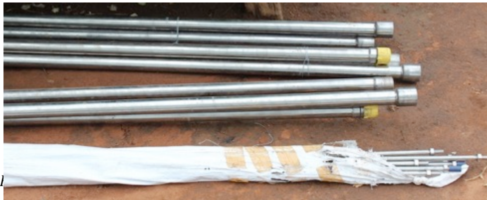
Figure 7. Stainless steel rising mains and rods used to rehabilitate two boreholes in Northern Uganda. Photo courtesy of Jake Carpenter.
