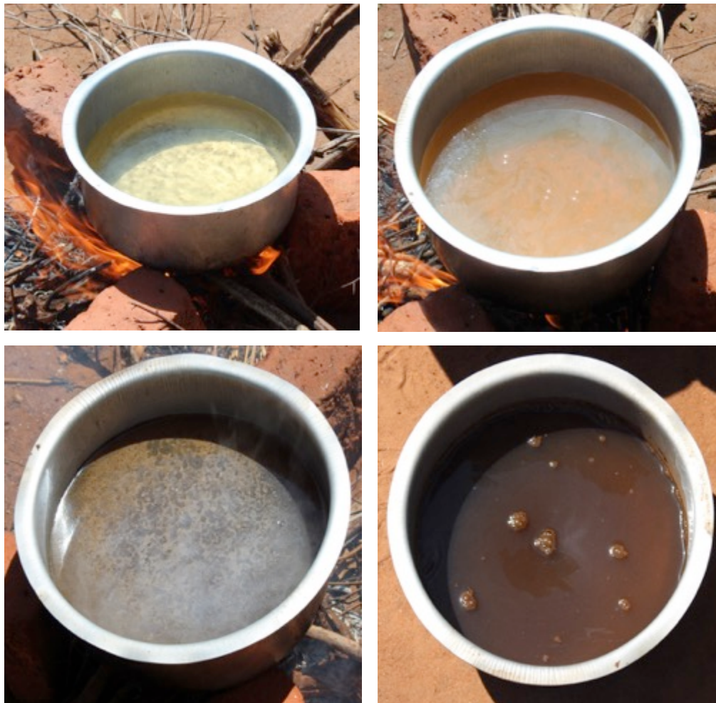
Figure 4. Water color of a sample of water taken from a Northern Uganda borehole progressively darkened as it was heated to a boil (left to right). The image in the fourth quadrant shows the state of the water once removed from the fire. The borehole has been chained up because the community did not deem the water acceptable for use. Many prefer collecting water from the unprotected spring. (Photos courtesy of Jake Carpenter)
