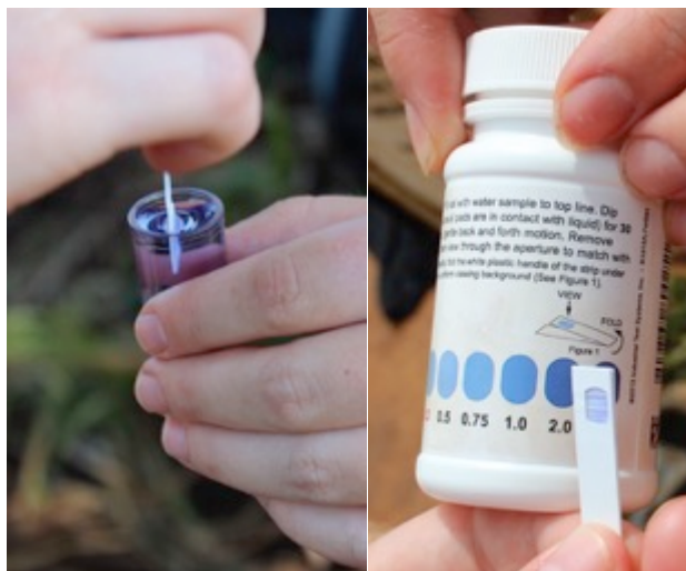
Figure 15. L: 30 seconds of gentle stirring followed by a 2-minute wait time with the strip removed from the sample. R: Matching strip to closest color on the container. (Photos courtesy of Jake Carpenter)
