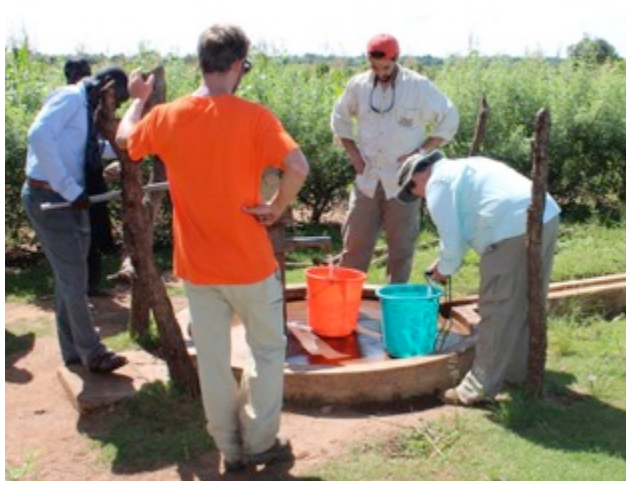
Figure 16. Measuring pH, conductivity, and TDS with the Hanna probe during a pump test at borehole 16.
