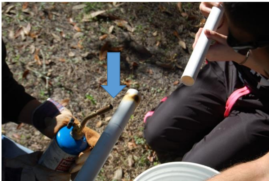
Figure 9. Heating a PVC Pipe
