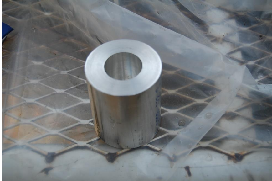
Figure 27. New Drive Cap for 0.75 in. Drive Pipe
