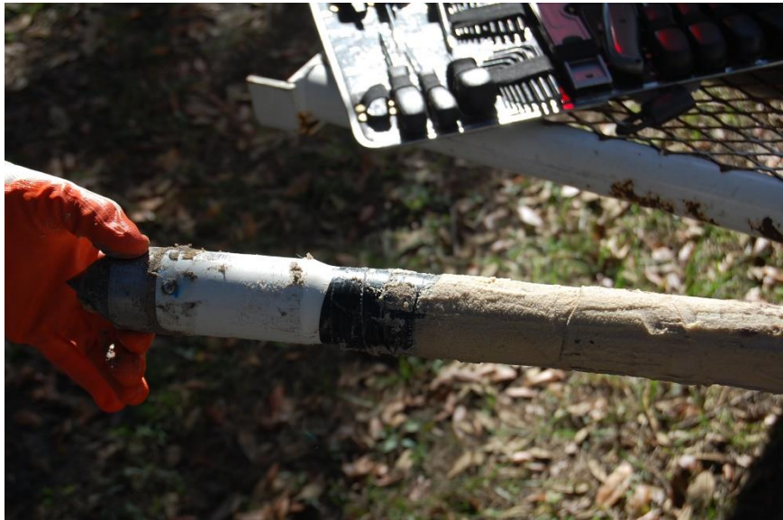
Figure 41. Exposed-Screen System B after Drilling Well #8
