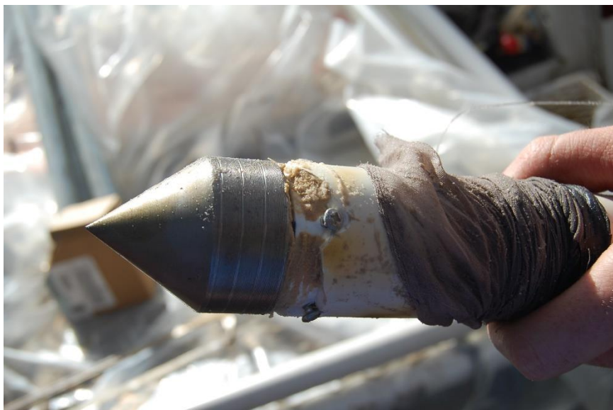
Figure 38. A Broken and Cracked Belled-End
