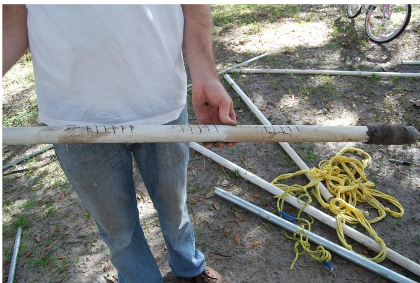
Figure 39. Sleeve Pulled Down on the Belled-End
