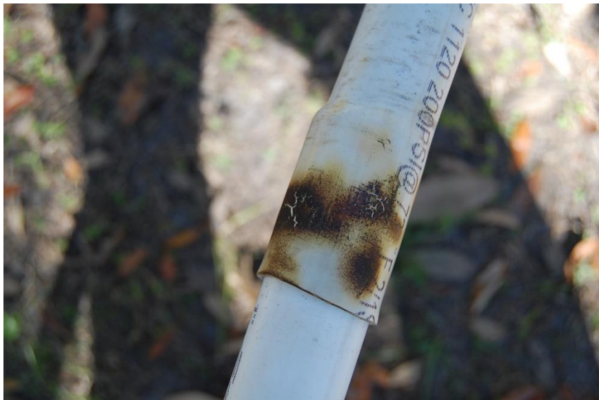
Figure 11. Final Result of Belling-Out a PVC Pipe
