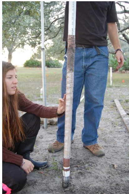
Figure 33. Exposed-Screen System A after Drilling
