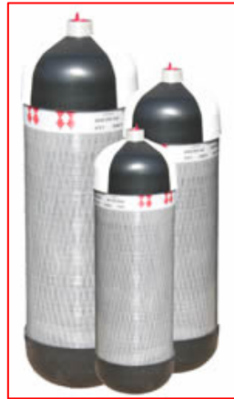
Type 2: Metal with composite hoop wrap
