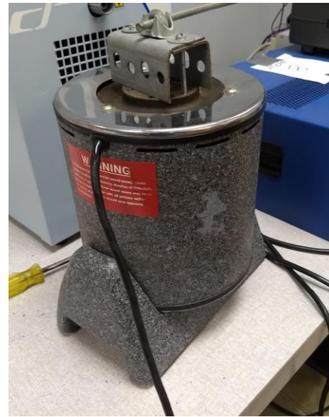
Figure 1: Shaker with cantilever rod assembly attached to output
