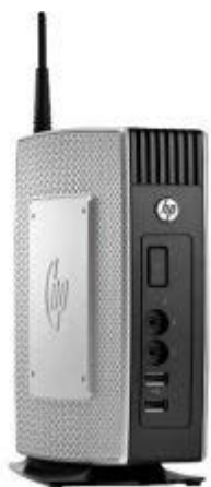
Figure 2.1.4 HP T5565. This thin client has a 1 GHZ processor, 1 GB of RAM, and costs $213.
