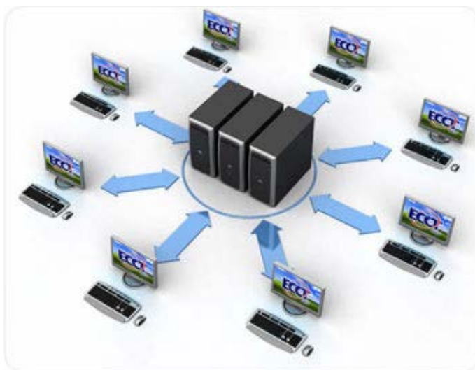
Figure 1. Network Diagram. A thin client PC network has one main server that does most of the computations for each thin client station.
