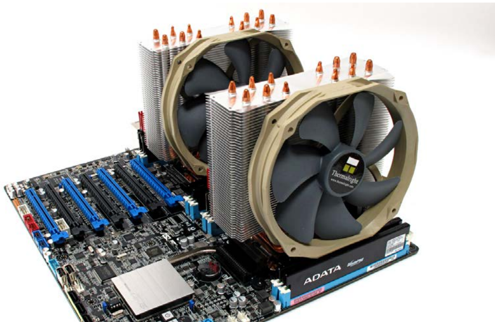
Figure 2.1.3: w Xeon E5-2690 processors sit on a high performance motherboard for greater processing power
