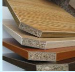
The resin used to hold layers/chips together contains HCHO
