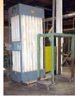
Aget Dust Collection Bag House $800 Model # FT-40 33" x 51" x 120" tall bag house 40 @ 5" dia. x 88" long bags 13" dia. air intake 240v or 460v 3 ph. shaker motor 37" x 58" x 72" welded steel stand No blower or cyclone
