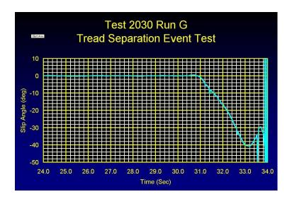
The next figure shows the vehicle's heading during the run. At approximately 31 seconds into the run, the vehicle violently changed: within one second, it jerked approximately 25 degrees; at two seconds, it changed directions by more than 50 degrees, and in less than three seconds the change in direction peaked at about 75 degrees.
