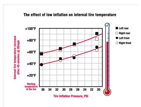
As depicted, with decreased inflation pressure, internal tire temperature increases after 45 minutes of operation at 85 mph.
