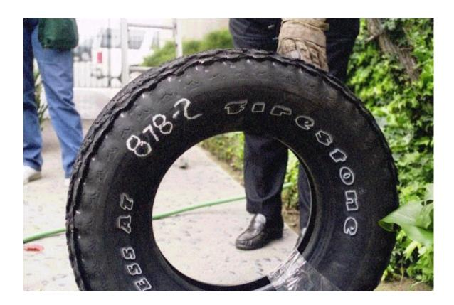
The testing was not designed to evaluate the durability of the tire. To the contrary, the testing was designed to evaluate certain force and moment characteristics of the tires in turning maneuvers. Although the test protocol requires severe slip angles in order to evaluate the performance capability of the tire in severe maneuvers, the tire should not fail during testing. This type of failure is further evidence of the lack of robustness present in the tires from a design standpoint.
