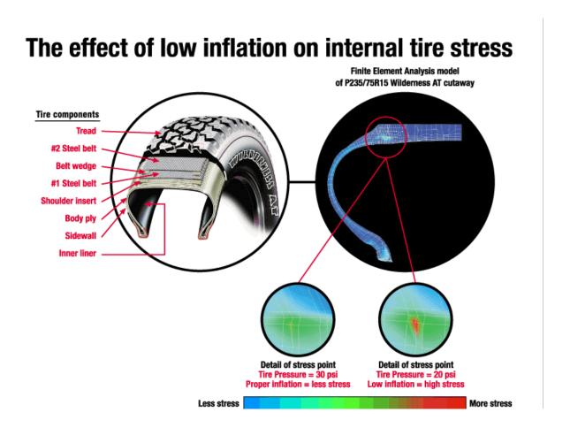
The effect of low inflation on internal tire temperature is illustrated by the following chart.
