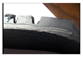
The cracks that start at the #2 belt edge result from a combination of a wedge that is poorly designed, both in its gauge and placement, a less-than-robust wedge compound, and a skim compound that is inadequate given the tire's other design characteristics.
