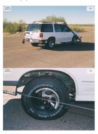
The test evaluated the vehicle's response to the simulated tread separation event. The steering wheel was held in a fixed position at 0±2 degrees, before and during the event, and the tread-separation event occurred over at least one second. The tests were videotaped.
