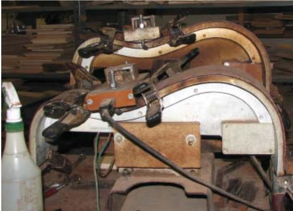
BENDING THE SIDES: Gradual hand pressure is applied to wet wood on a hot bending template to shape the sides of guitars.
