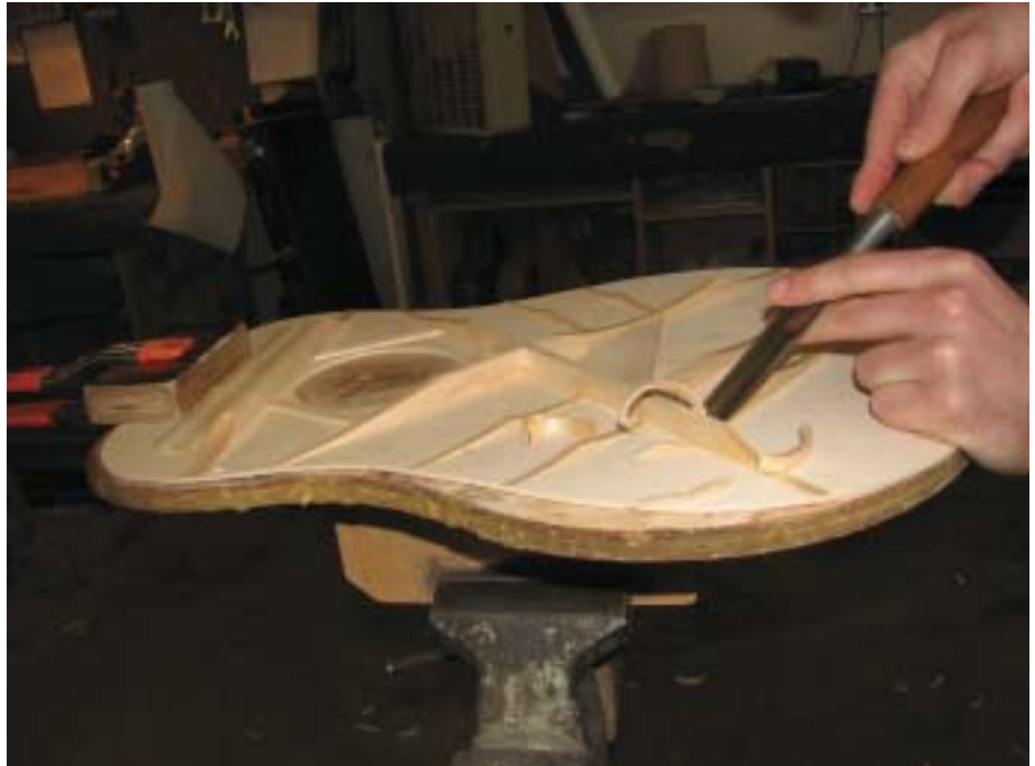
SHAVING THE BRACES: The thickness of the guitar's top and braces influence a guitar's sound, so the luthier listens to the tone that develops after a series of ribbons of wood are shaved off the braces.
