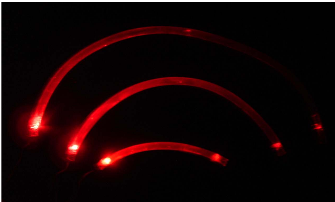
Figure 14: Picture of Red LED Gel Tube Transmission along Curved Path
