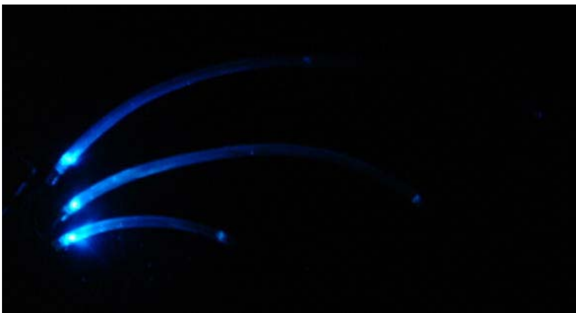
Figure 25: Picture of Blue LED Gel Tube Transmission along Straight Path
