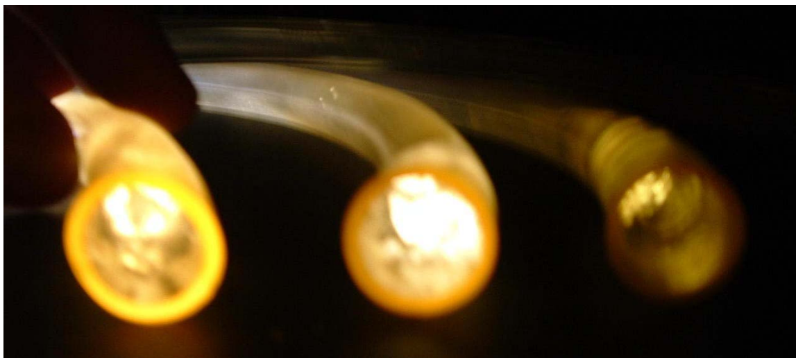
Figure 21: Picture of Output Spectral Intensity of White LED for One-, Two-, and Three-foot Gel Tubes
