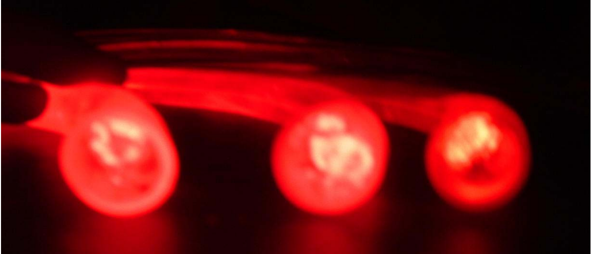
Figure 16: Picture of Output Spectral Intensity of Red LED for One-, Two-, and Three-foot Gel Tubes
