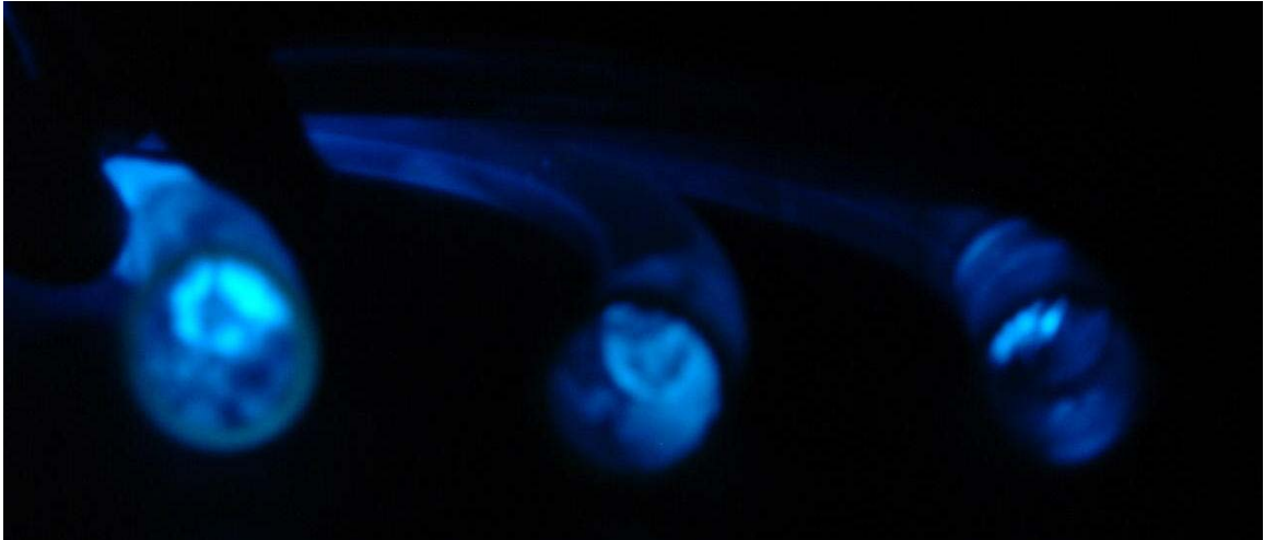
Figure 26: Picture of Output Spectral Intensity of Blue LED for One-, Two-, and Three-foot Gel Tubes
